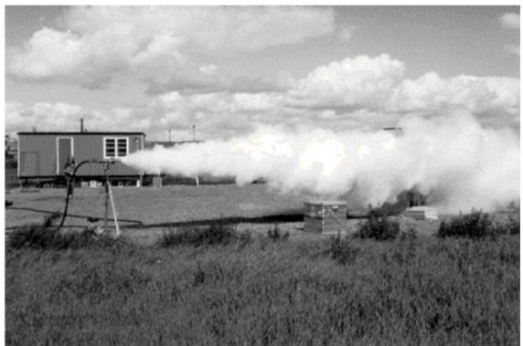
Fig. 2. Photograph of one of the FLADIS ammonia trials, kindly provided to HSE by Morten Nielsen (DTU). The ammonia jet source is 1.5 m above the ground.
