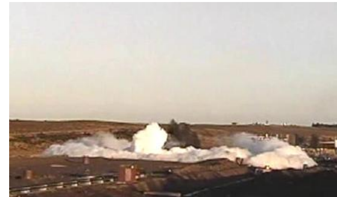
Plume fountain falls back on itself, CO 2 re-entrained, dense blanket formed
