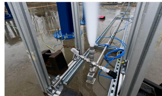
Nozzle and release system commissioning
